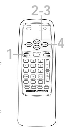
Press the PLAY/▲ button or the STOP/▼ button to select SET PBS CH. MANUAL. Then, press the F.FWD/ **button**. The default channel (02) flashes.
